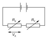
The variable resistors have resistances  $R_X$  and  $R_Y$ .  $V_X$  is the potential difference across resistance  $R_X$ .
